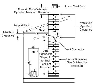
Venting Through Chimney With Type B Double Wall Vent Pipe.
